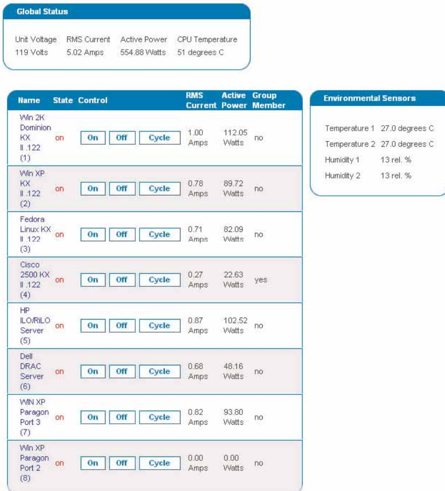
An example of a Web browser GUI showing outlet switching, outlet metering and environmental information.
