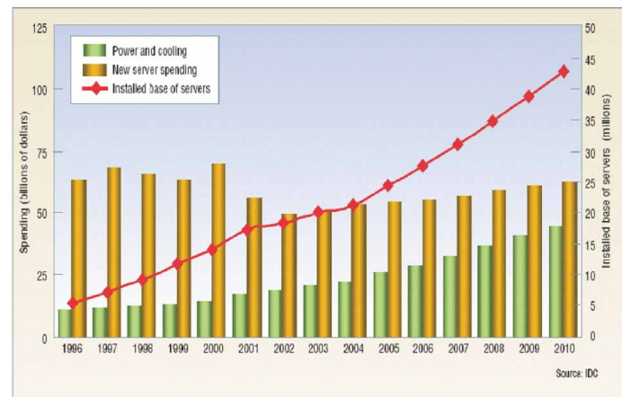
Although new server spending is leveling off, the industry is experiencing double-digit increases in server density, with a corresponding increase in the demand for power and cooling. (Source: IDC)
